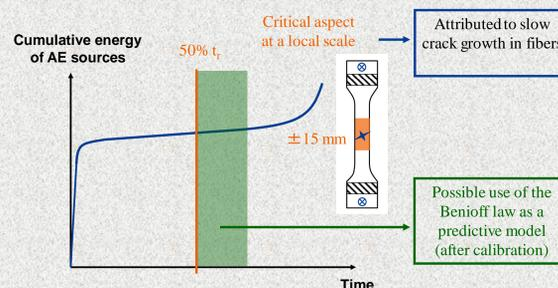
A criterion denoted  $R_{AE}$  was defined, which allows prediction of the time-to-rupture using AE activity recorded during the first half of the test. This criterion is a reliable indicator of the beginning of a new damage stage leading to ultimate fracture.
