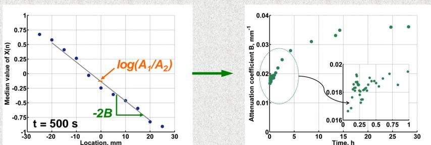
For ceramic matrix composites under static fatigue loading, a significant increase of energy attenuation is observed during the first half of tests. This increase of attenuation is associated to transverse matrix crack opening.
